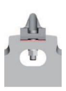
Shimplates should be fitted when the chain is lengthened due to wear by apprx. 2,5%. The replacement of the chain is recommended with the quality grade E10 by a chain wear of apprx. 3,5% and quality grade E14 by 5%.
